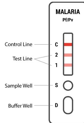
Absence of a coloured band in the test region indicates a non-reactive test result. A procedural control line should always develop at the 'C' region to indicate that the test has been carried out correctly.
